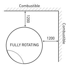
950mm minimum clearance is required if the rotation of the BathyscaFocus is locked at 120° or 90° away from the wall. Locking the BathyscaFocus so that the opening is fixed is an option available on purchase.
